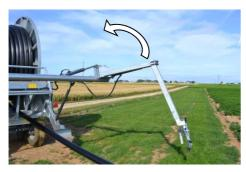
After laying down the PE-pipe open the fairlead and lift up the swivel arm in order to clear the space for the cart.
