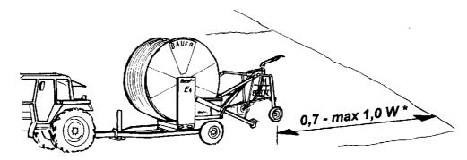
Drive into the field with the Rainstar considering the trajectory of the sprinkler.
