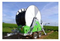
Lower the supports with the hydraulic control on the left and on the right side equally.
