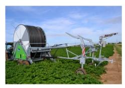
Lower the cart with the hydraulic cart lift and fix it to the ground.
